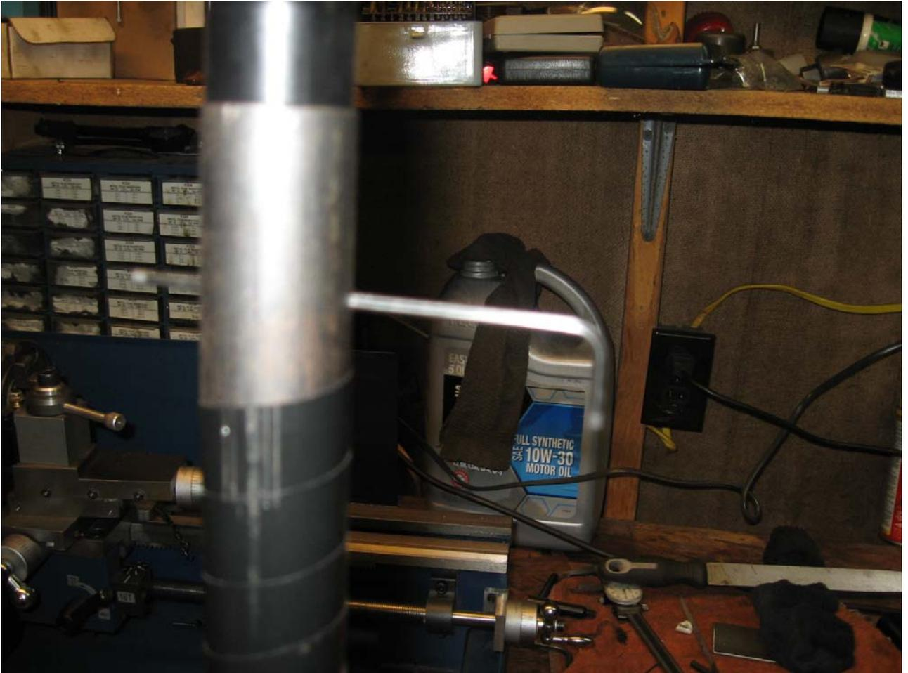
You can now drive the 1/8" compression pin all the way in using your metal hammer. Yes I said you can use your metal hammer now. Drive it flush with the surface of the bar and your FINISHED.
