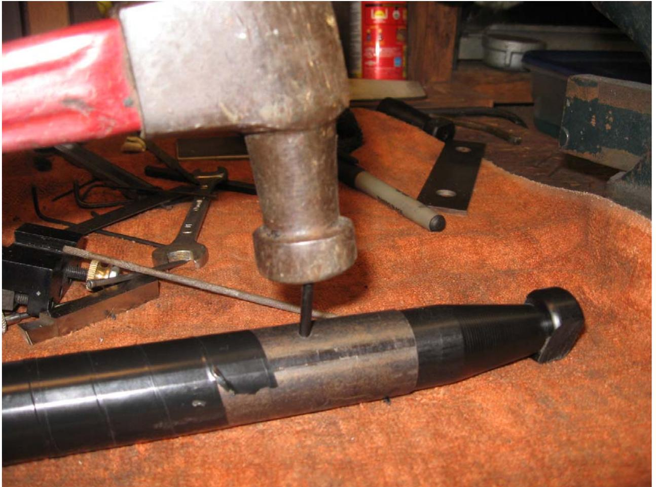
Here is the finished product. Note the orientation of the black mark on the top of the 5/16" hardened steel rod in relation to the 1/8" hole that is offset slightly to the left. This is really a simple process as long as you take your time and think about what your doing before you do it. Also notice that the 5/16" hardened steel rod is raised slightly above the end of the bobbin.
