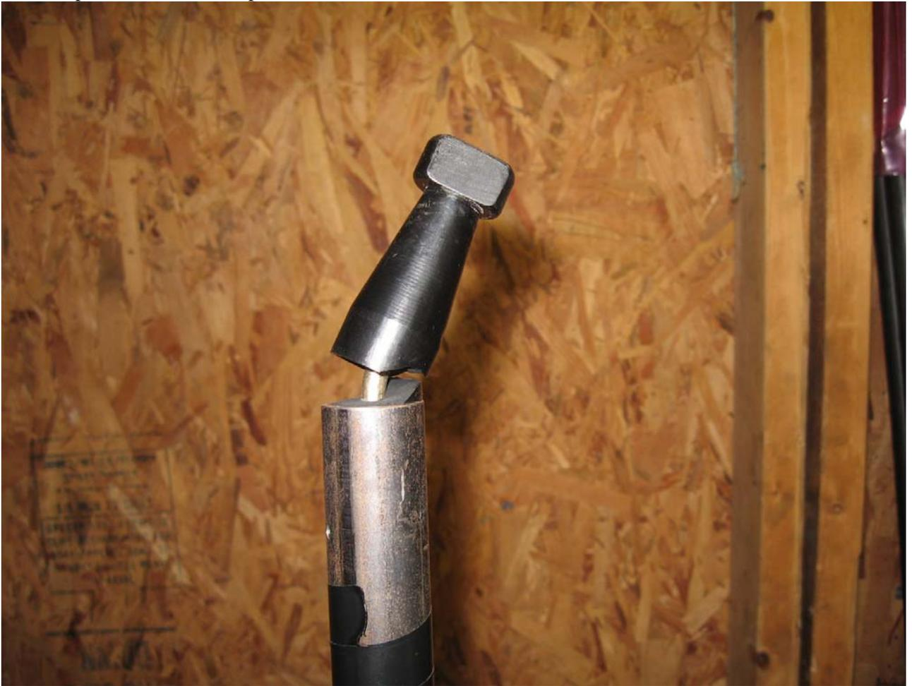
The first step in replacing your demount tip is to knock out the 1/8" compression pin which holds the tip in place. Please don't try to fit a 3/16" long round object in a 1/8" hole. I use an old jeweler's file that I broke doing something with it I shouldn't have. Knock it all the way out and be sure to save the pin. You can now remove the hardened steel rod along with whatever remains are left of the delrin tip.
