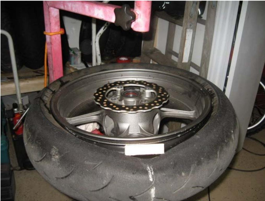
Now insert the demount end of the tool with one of the flat sides facing the rim and the other facing the lip of the tire as shown below. You should use a shot of silicon on the demount tip as a precaution to avoid scratching the rim. Spray the silicon on the demount tip for demounting both beads of the tire.
