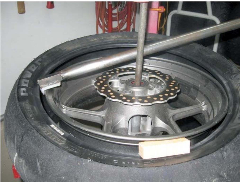
Make sure the bead of tire is on top of the right lip of the mount end. This will take a bit of effort to get it right but the tool will NOT work if this step is not done properly.
