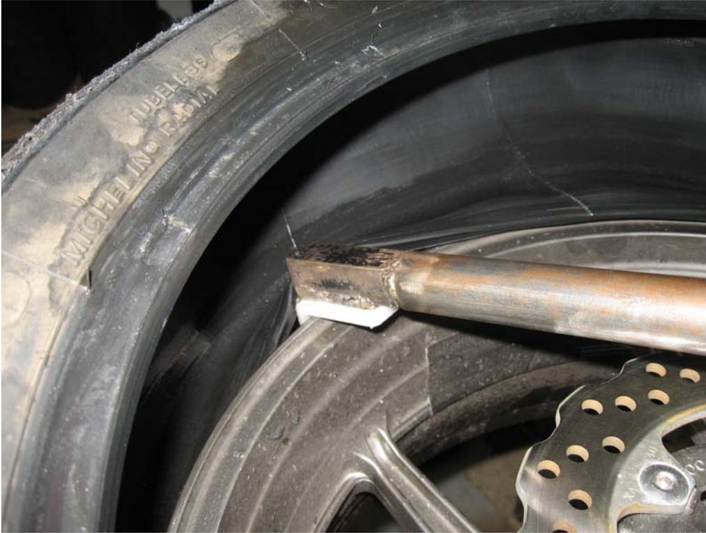
Again use the block of wood to hold the bead of the tire in the **CENTER** of the rim.
