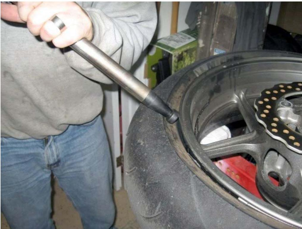
After the demount tip is inserted between the rim and the tire, rotate the tool 90 degrees so the lip of the demount tip catches the bead of the tire and lift up the tire bead. See my **Demount tip replacement document** for what happens if you don't lift the tire bead up.
