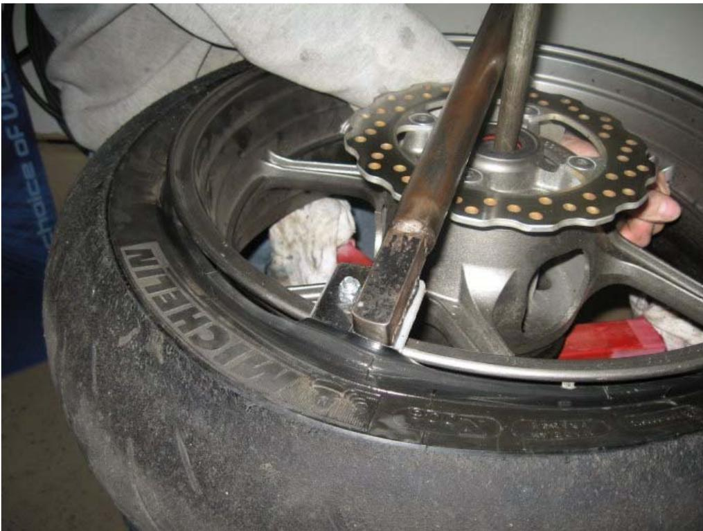
The last step is to lift the tire tool vertically to seat the remaining couple inches of the tire bead on the rim.
