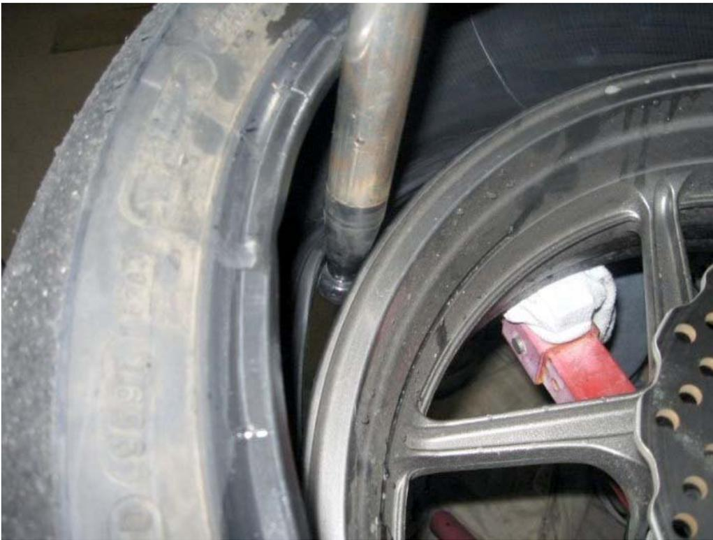
Make sure you liberally lubricate both sides of the tire before mounting. Be sure to lubricate the **INSIDE** of both beads as well. Also make sure you wipe any excess lubricant out of the inside of the tire. It will make balancing difficult if you leave excess lubricant inside the tire.
