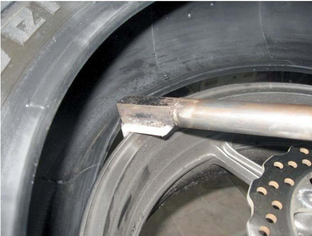
Now rotate the tire tool in the **CLOCKWISE** direction until the first bead drops over the rim. On some tires with enough lubricate you don't need to use the mount end but can muscle the first bead over the rim. **It's all in the technique when trying the above.**
