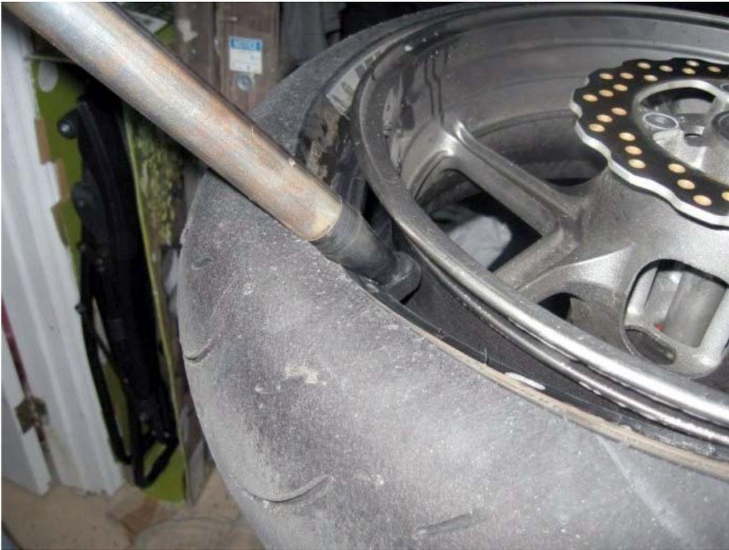
Now move the tire tool to the position below making sure that the opposite side of the tire is in the CENTER (smaller) part of the rim.
