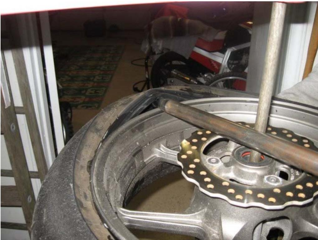
Rotate the tire tool either clockwise or counter clockwise depending on which side of the vertical leverage bar the tire tool is resting. In the above picture note that the tire tool is on the left side of the vertical bar so you need to rotate the tool counter clockwise. Rotate the tire tool until the top bead of the tire is completely free from the rim.
